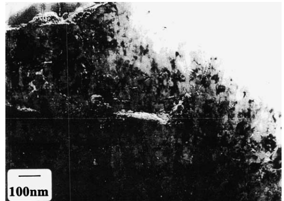
Fig. 14. Underfocus image of section of thin oxide on Zr-2.5% Nb showing lateral cracks only adjacent to the perforation resulting from ion-milling [56].
